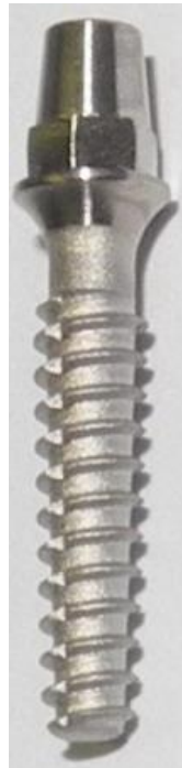
Scheme of implant from nanostructured Ti, (d) Prototype model of 2.2 mm-implant
